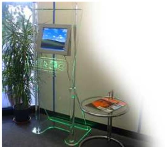
Slim-Line Glass Floor standing kiosk with 15" VIA 1Ghz Panel PC
