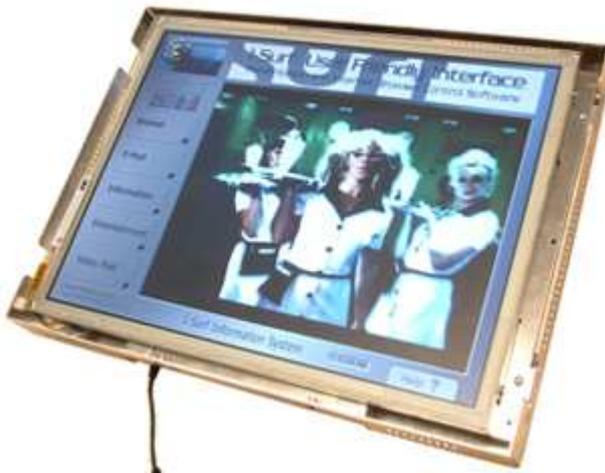
15" Screen Multi-Media Kiosk Panel PC with Fanless 1 GHz VIA Industrial M/Board, 256 Mb RAM, 40 Gb HDD and Windows O/S
